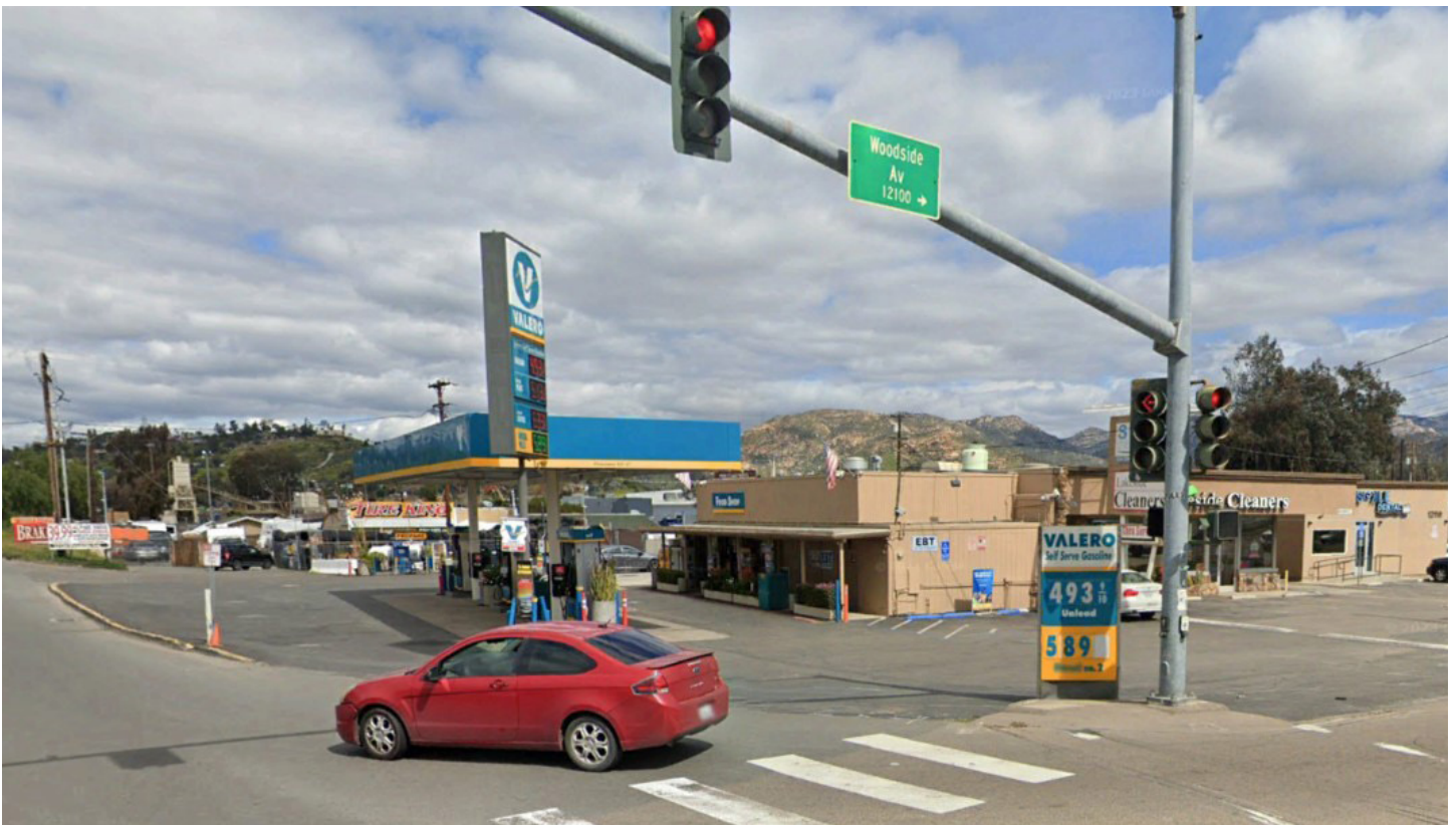
Missing pedestrian facility - signalized intersection has no connection with sidewalk or landing
